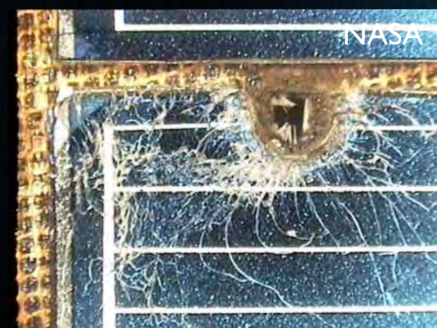
4 cm hole in the solar panel on Hubble
